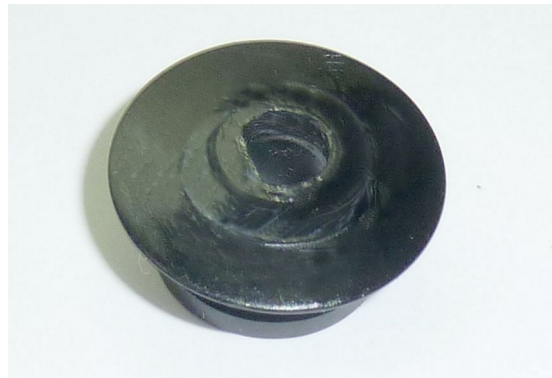
Washer glued in place in bush
